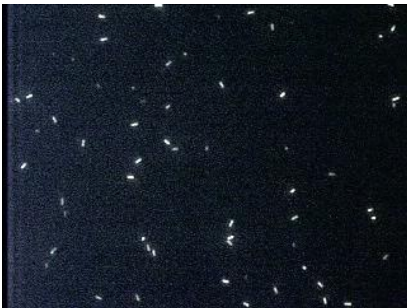
Pt/Au rods in \text{H}_2\text{O} (DI)
