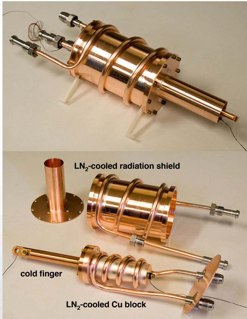
Simple LN 2 cooling coil cryostat with flex links for condensing Kr samples at 117.5 K
