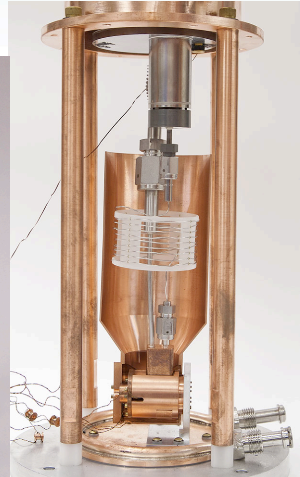
Capillary flow impedance and pumping line connections
