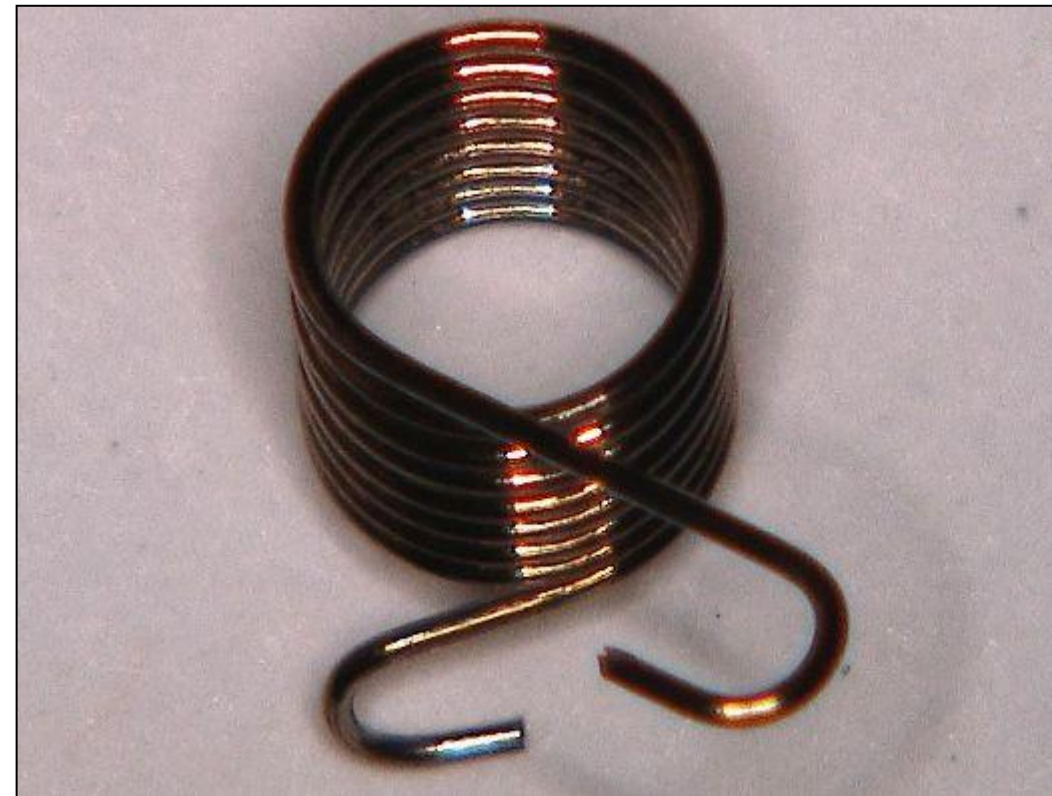
FIGURE 1. An Elgiloy meso-scale torsion spring with 0.175mm wire diameter, 3.8mm spring length and 2.5mm coil diameter.
