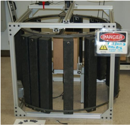
Figure 1: Photograph of the prototype time encoded imager. The 5" diameter LOS cell is inside the box at the center.
