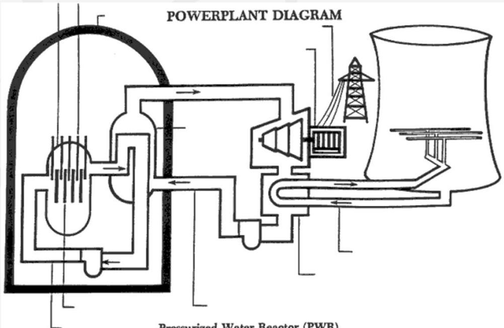
Pressurized Water Reactor (PWR)
