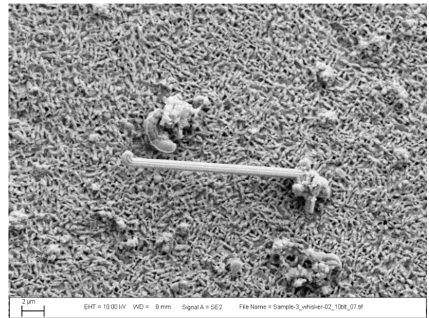
Figure 2. SEM examples of straight, kinked, and curved whiskers, and a whisker that subsequently grew as a hillock or "odd-shaped eruption".
