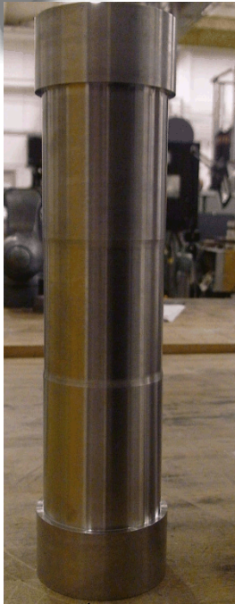
3" Reduced section, from 0.050" to 0.020"
