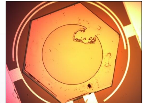
Assembled triple junction microsolar cell with decoupled connections
