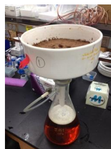
Poplar wood chips pretreated in the steam reactor to form biomass suitable for biofuel production.
