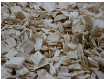
Poplar wood chips pretreated in the steam reactor to form biomass suitable for biofuel production.
