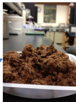
Poplar wood chips pretreated in the steam reactor to form biomass suitable for biofuel production.
