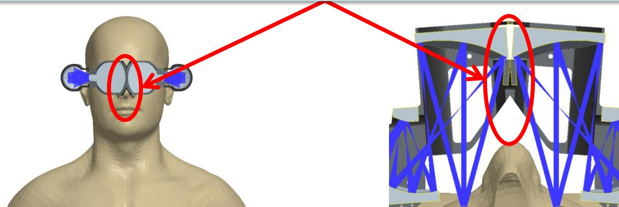
Reduced pupil (2.5mm vs. 3.0mm) design allows for some space between the two assemblies
