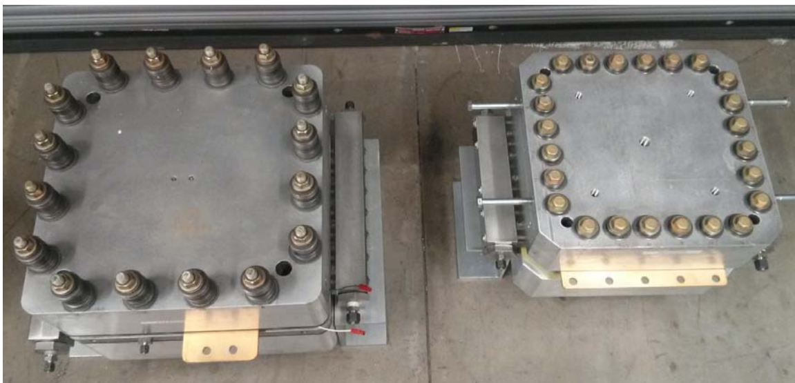
Figure 83: Legacy Stack vs. 40% Cost-Reduced Stack (20% Larger Active Area)
