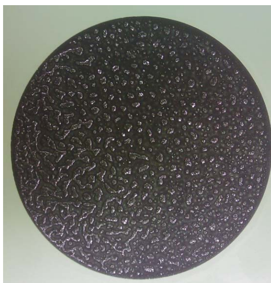
Figure 14: Printed Ink Decal Showing Bubble Agglomerates
