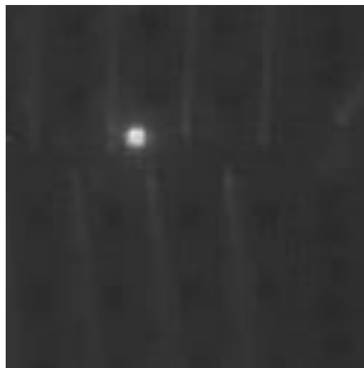
Figure 10. A single frame from an AVI file showing emission from a single 50 x 50 \mu\text{m}^2 photonic emitter tuned to an MWIR band.
