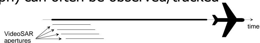
A rapid sequence of SAR images (> 1 Hz) can permit observation of target shadows
