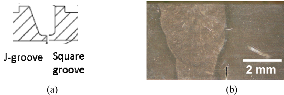
Figure 7 (a) Modified weld joint design of J-groove coupled with square-groove for GTA welding. (b) GTA weld etched to reveal FZ and BM with machined notch positioned on square-groove side of weld joint. FZ/BM interface appears to be close to parallel to notch and crack growth plane.
