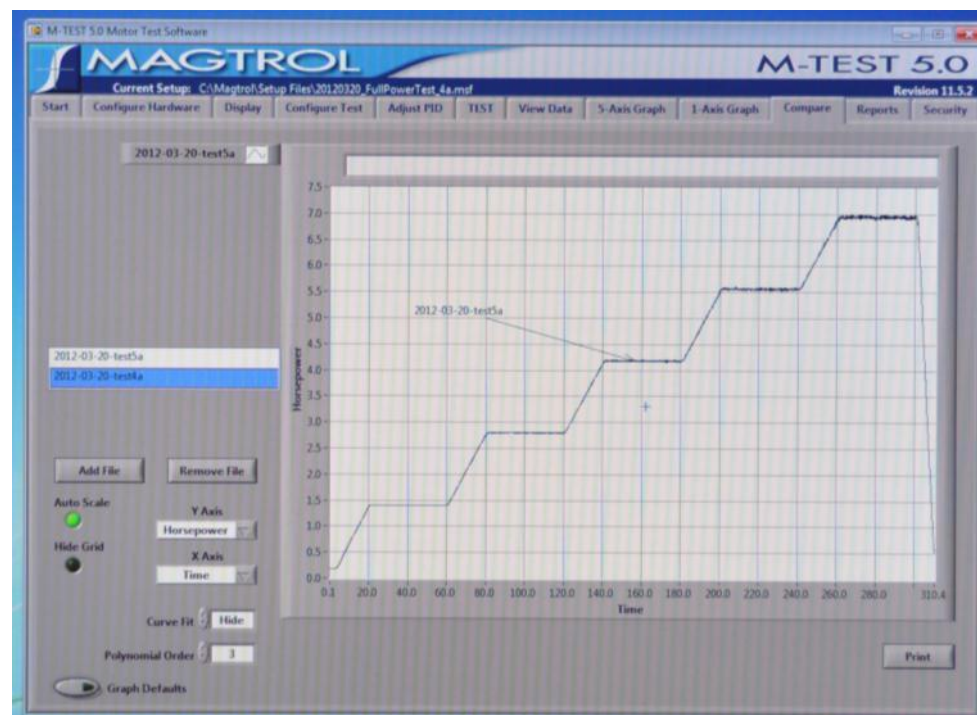
Dynamometer Testing Load Profile (Torque vs. Time)
