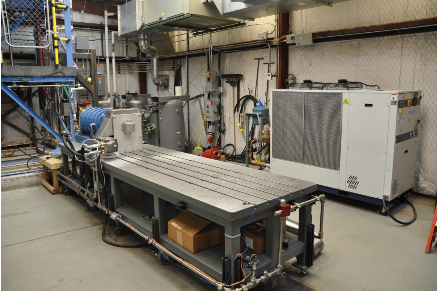
Dynamometer Test Station (DTS) – configured for dynamometer verification testing
