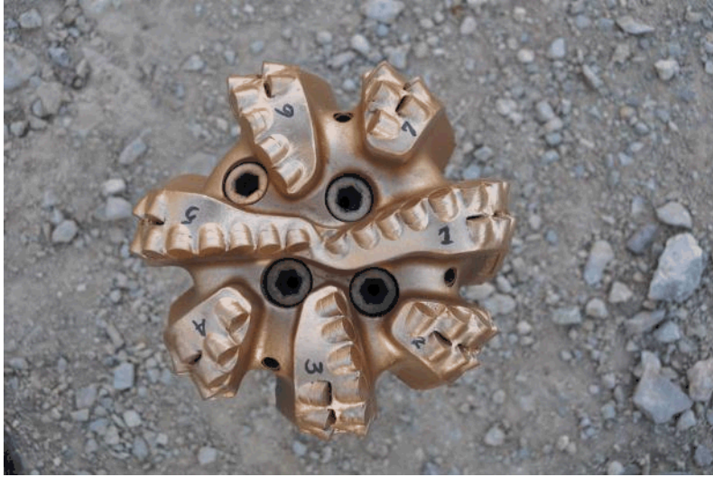
Bit 2A: Pre-Drill Sharp Condition
