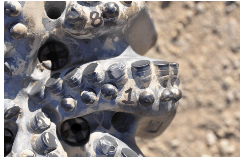
Bit 1A after drilling showing minor cutter damage
