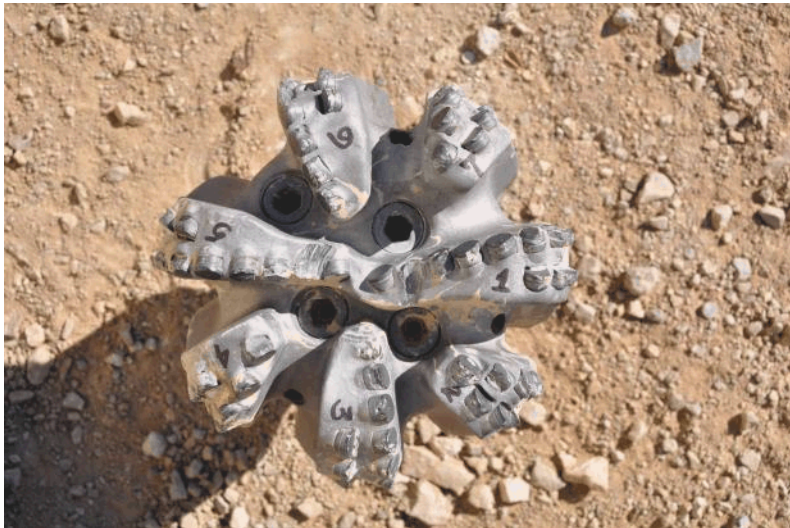
Bit 2A: Post Drill Condition (after 566 ft.)
