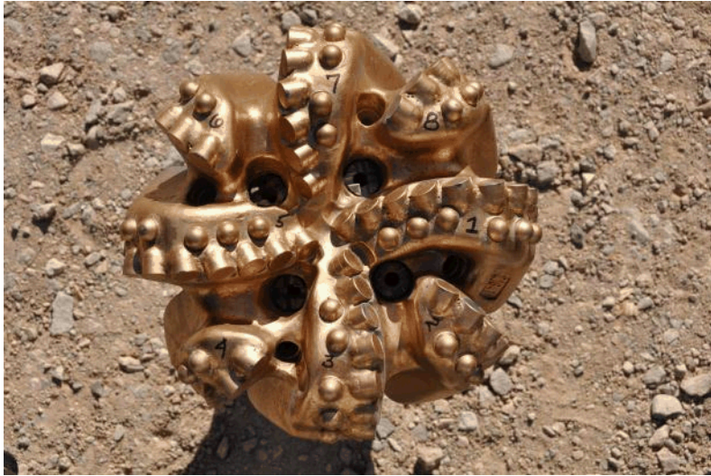
Bit 1A: Pre-Drill Sharp Condition
