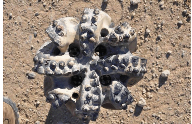
Bit 1A: Post Drill Condition (after 725 ft.)
