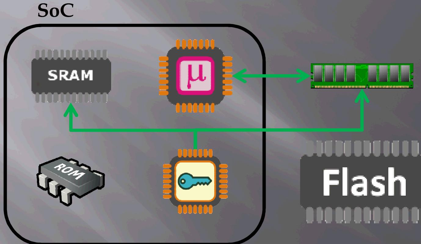
The resulting decrypted bootloader is then loaded into either SRAM or standard DRAM and execution continues.
