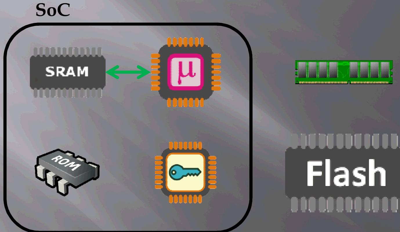
Next, the microprocessor begins execution out of the secure RAM.
