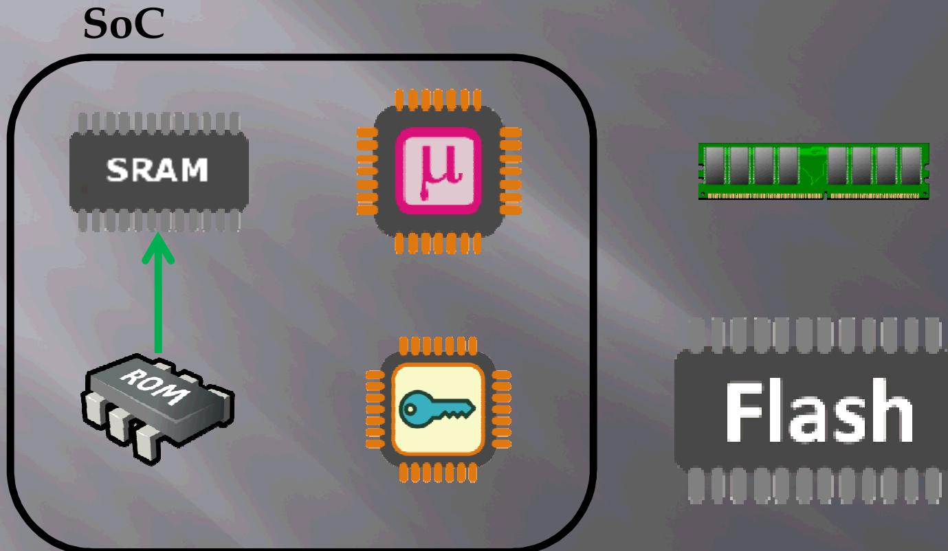
The first step is pulling the boot-rom from some form of read-only memory and loading it into secure RAM.
