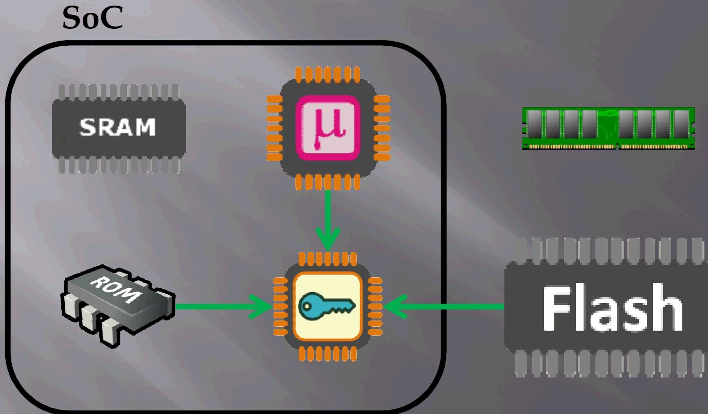
The microprocessor then sends a command to the crypto engine to retrieve a secret key from some form of ROM and decrypt the 1<sup>st</sup> stage bootloader from flash.
