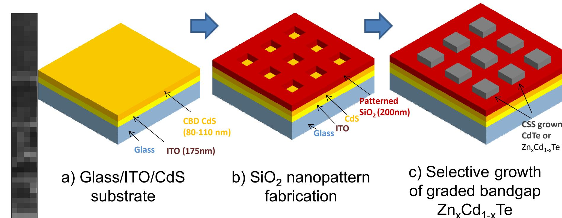
Five methods were successfully tried to create the nanopattern. Standard lithography (2  $\mu$ m) and step and flash imprint lithography (280 nm) were used for CdTe growths. The pattern was transferred on the PECVD grown SiO<sub>2</sub> with a CHF<sub>3</sub> etch.
