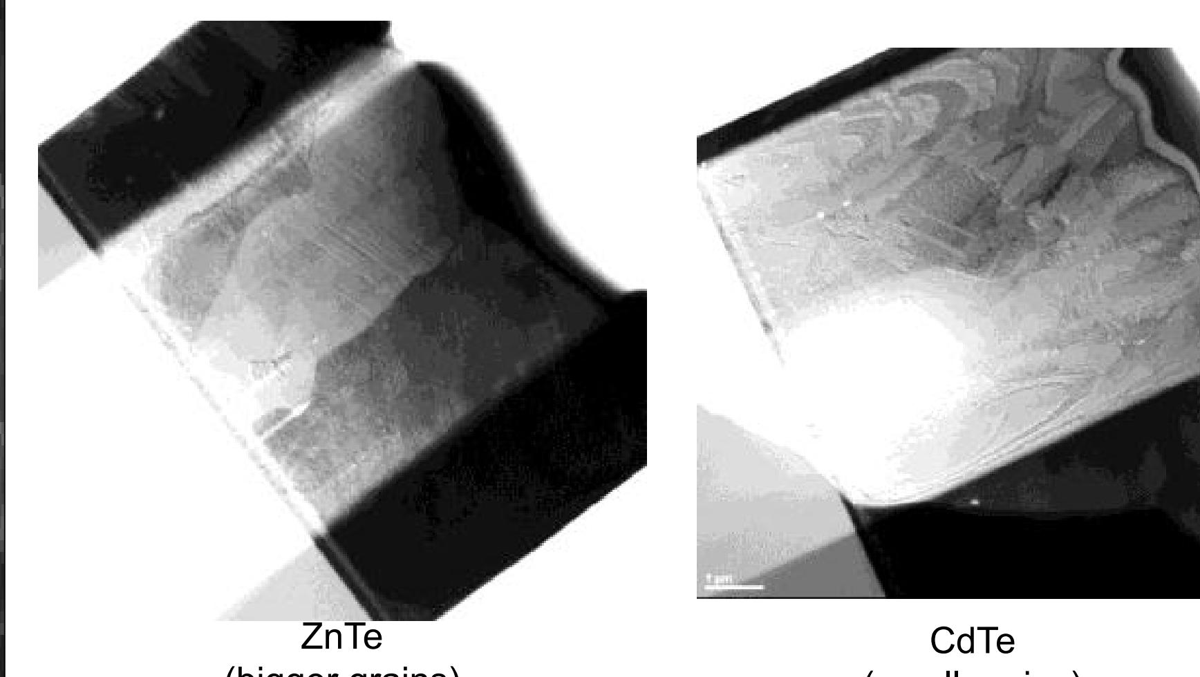
TEM cross-section image of CdTe/ZnTe deposited on CdS and CdTe deposited on CdS. The TEM shows that introducing ZnTe yields larger grains
