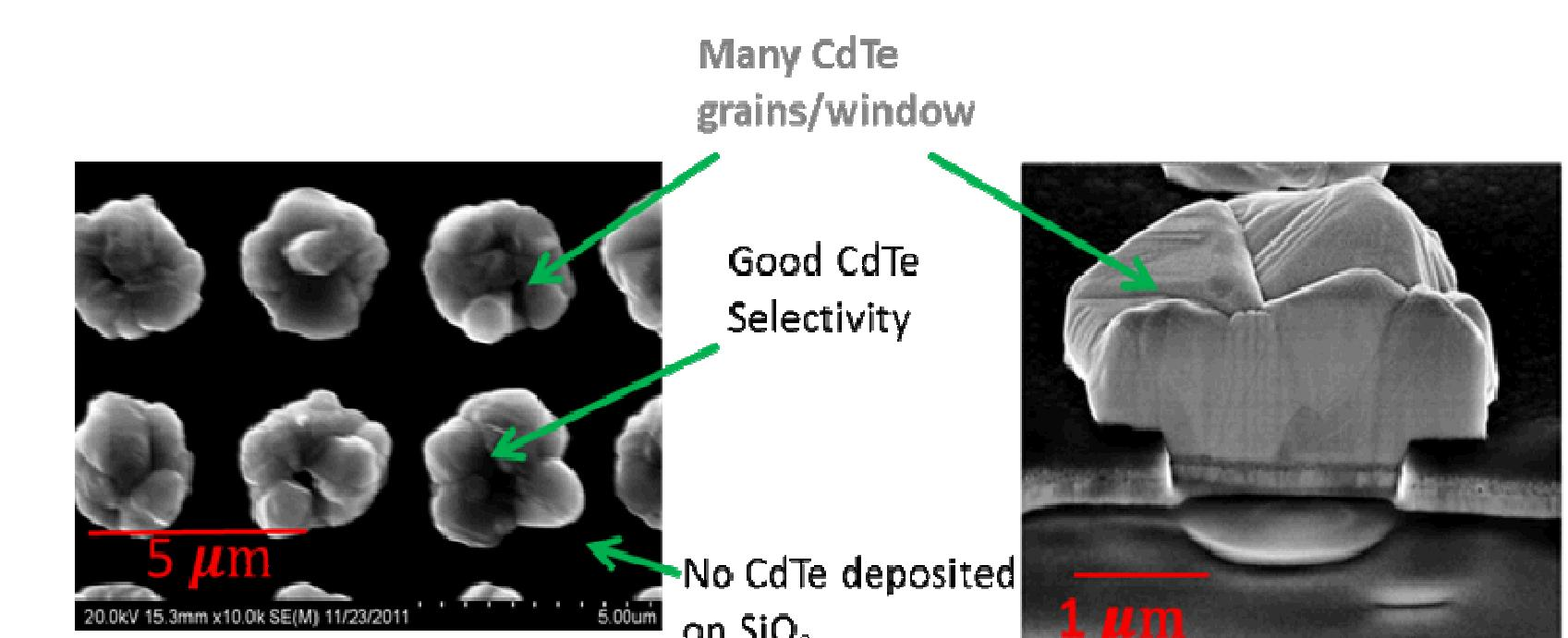
Top and cross-section SEM images of CdTe selective growth on 2  $\mu$ m-window size glass/ITO/CdS patterned substrates
