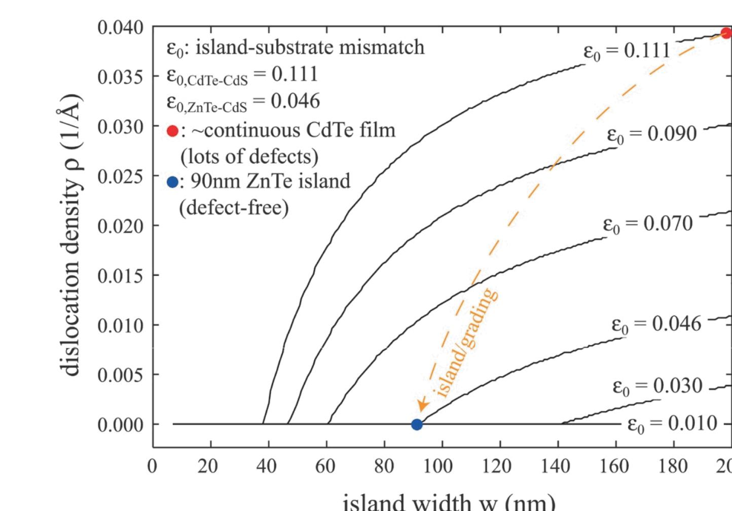
Dislocation density as a function of window size for different CdTe-CdS and ZnTe-CdS island-substrate mismatch. Dislocation density is predicted to be reduced substantially by using the island growth with graded material.
