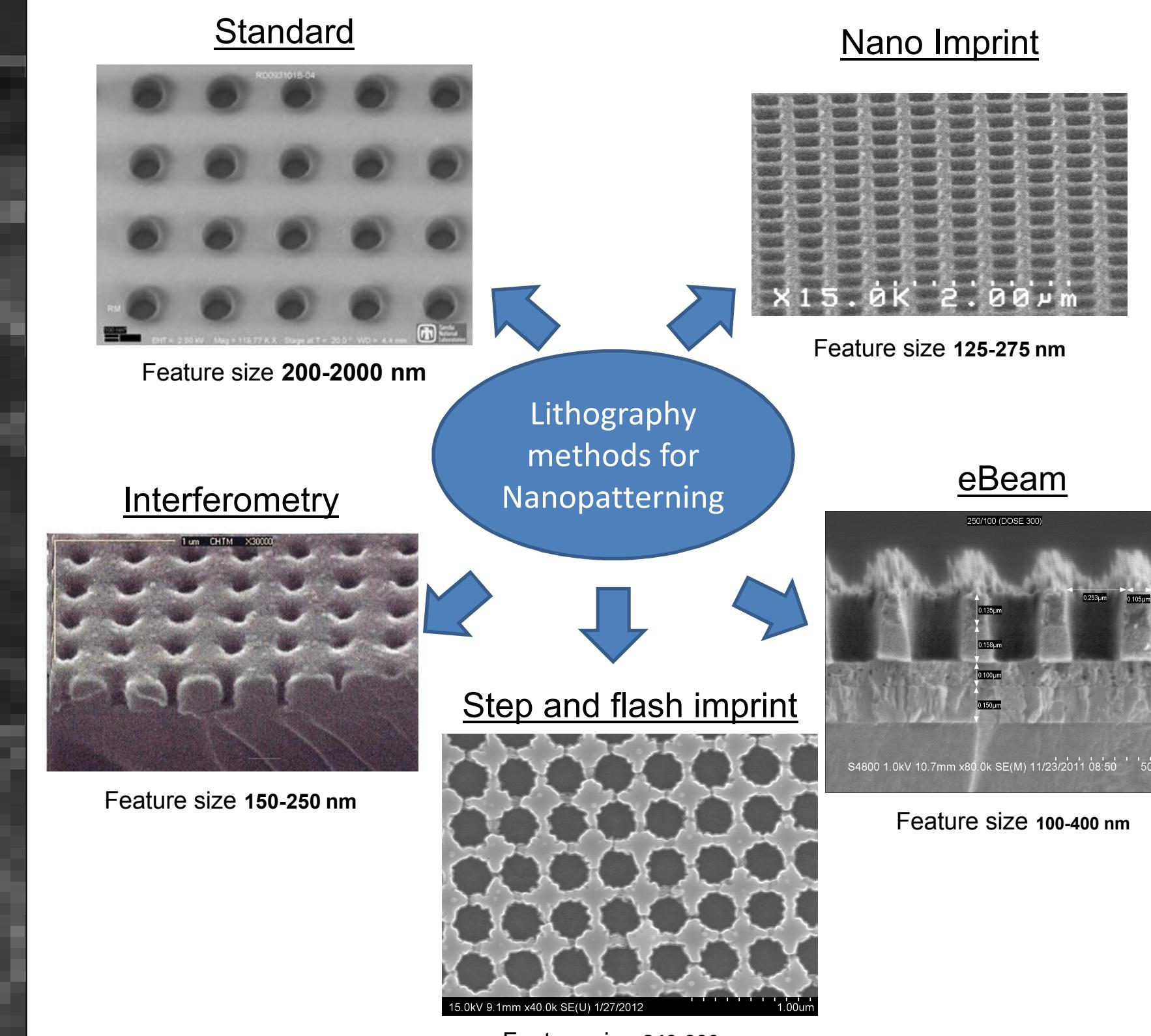
SEM pictures of nanopatterned substrates obtained by different techniques to be used as templates for selective growth
