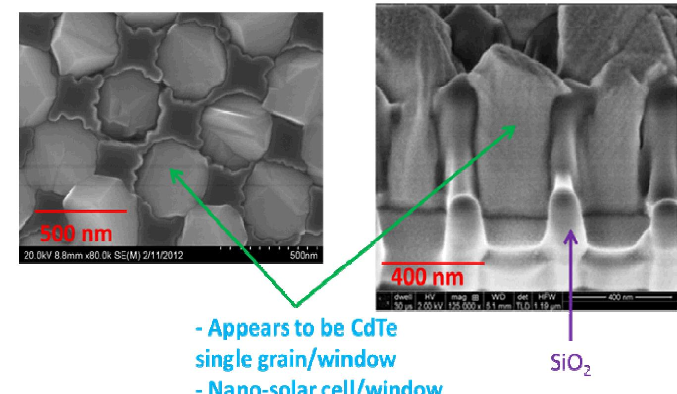
Top and cross-section SEM images of CdTe selective growth on 285 nm window size glass/ITO/CdS patterned substrates. In comparison with the micro pattern, the nanopattern seems to generate single grains per window.
