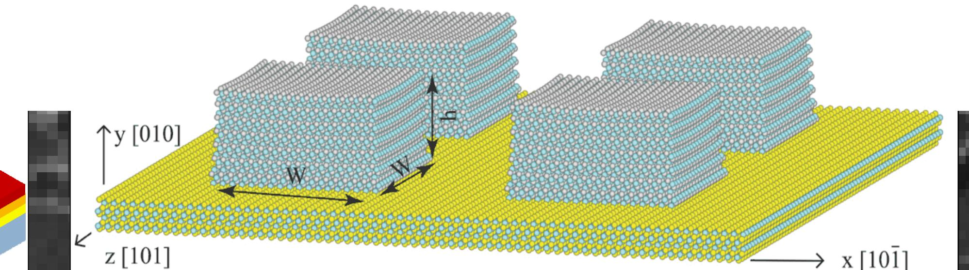
Simulated growth of nanoislands of CdTe on CdS. The stress due to lattice mismatch relaxes as the structure grows.
