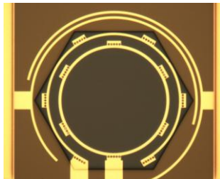
Fig. 5 a) shows the overlay of the photolithography masks used to create the c-Si PV cell (receiving substrate) where each color describes one mask. Fig. 5b) is a microscope image of the front of the c-Si PV cell.
