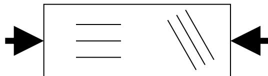
An in-plane compressive force develops because  $\text{ErT}_2$  grains wish to expand but the film geometry limits this. Out-of-plane expansion is not likewise hindered.
