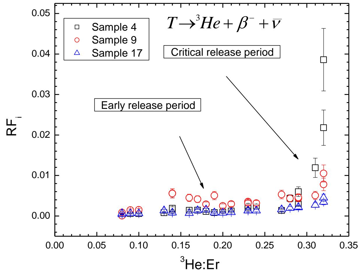
Typical  ${}^3\text{He}$  release characteristics indicate most  ${}^3\text{He}$  generated remains in lattice.
