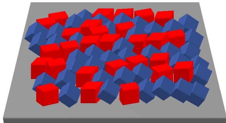
Schematic showing a *bi-modal* (111) and (200) out-of-plane preferred orientation for  $\text{ErT}_2$  grains.
