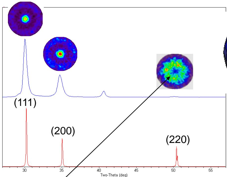
Ring of intensity in the  $\text{ErT}_2$  (220) Pole-figure is critical for accurate diagnosis of texture
