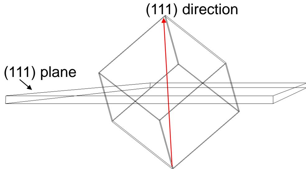
${}^3\text{He}$  bubbles are long thin plates that propagate along the (111) planes in the Fluorite-type  $\text{ErT}_2$  lattice
