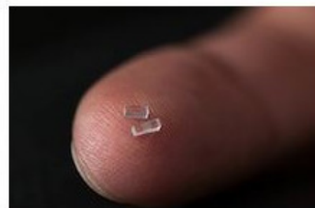
Nanofabricated chips of fused silica just 3 millimeters long were used to accelerate electrons at a rate 10 times higher than conventional particle accelerator technology. (Brad Plummer/SLAC)
