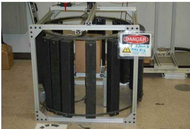
Figure 1: Left: The LIGHTHOUSE detector built from a rotating mask of High Density Polyethylene (HDPE) with a single 5” liquid scintillator cell and photo-multiplier tube (PMT) in the center. Right: The PRISM detector consisting of three large cells each housing liquid scintillator and a 9” PMT rotating on a central axis.
