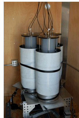
Figure 1: Left: The LIGHTHOUSE detector built from a rotating mask of High Density Polyethylene (HDPE) with a single 5” liquid scintillator cell and photo-multiplier tube (PMT) in the center. Right: The PRISM detector consisting of three large cells each housing liquid scintillator and a 9” PMT rotating on a central axis.
