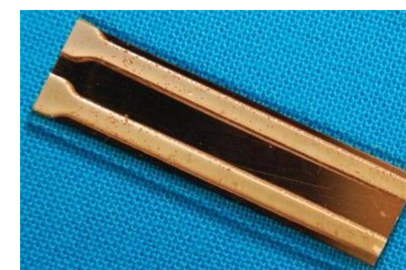
Photograph of a 100 μm thick HNAB lines confined by 4 μm copper layers on a 1 cm x 3 cm Lexan substrate. Films are patterned in this geometry for use in detonation experiments
