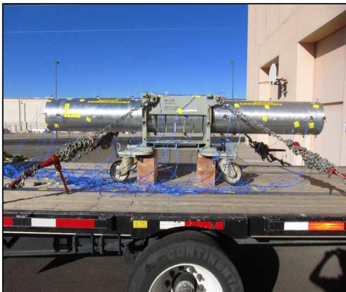
Instrumentation Layout for Simulator
