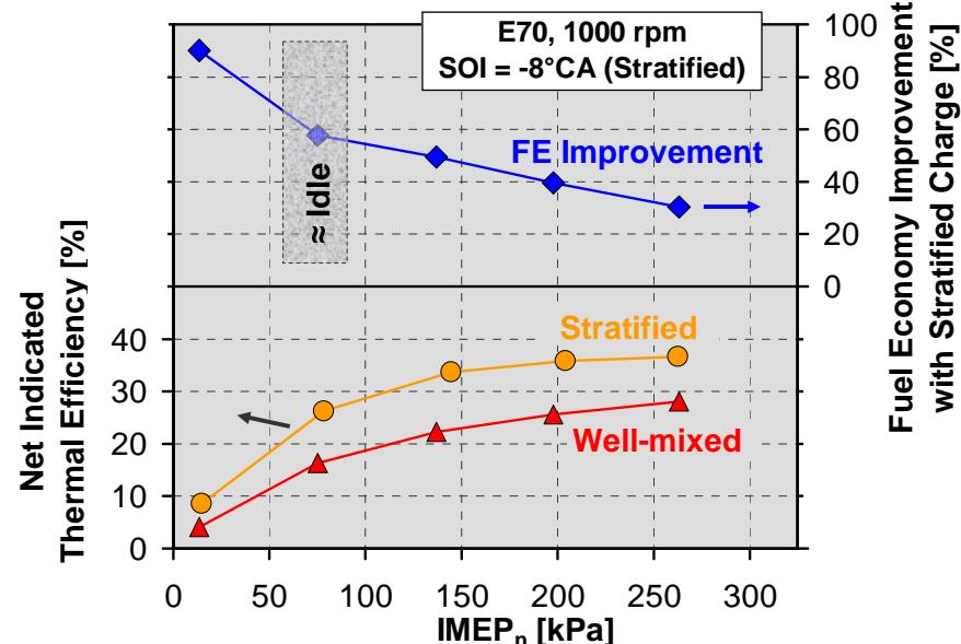
**Objective:** Characterize the combustion mode with near-TDC injection of E85.
