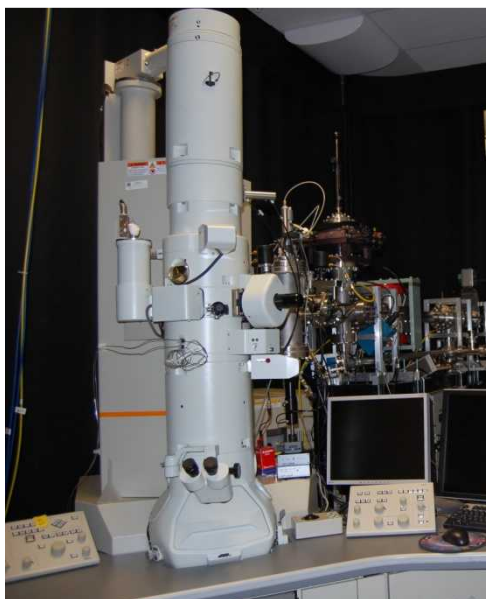
Figure 2: I^3 TEM with beamline from 6 MV Tandem Accelerator coming into the TEM perpendicular to the column.
