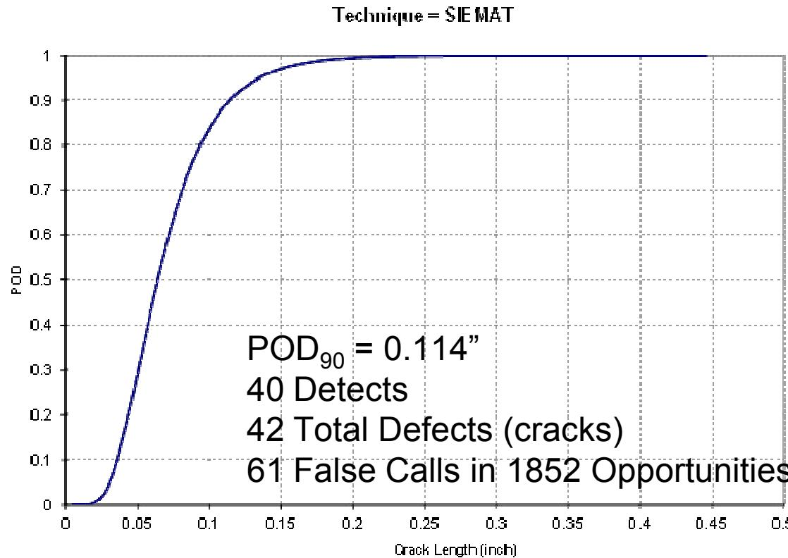
POD calculated using Spencer's Multi-Flaw Model (which takes into account the possibility of more than one defect at each independent inspection location) with a 2-parameter probit model fit of hit/miss data.
