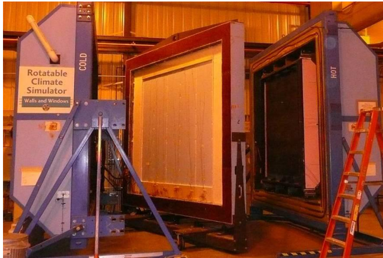
Figure 3. ORNL Rotatable Guarded Hot Box.
