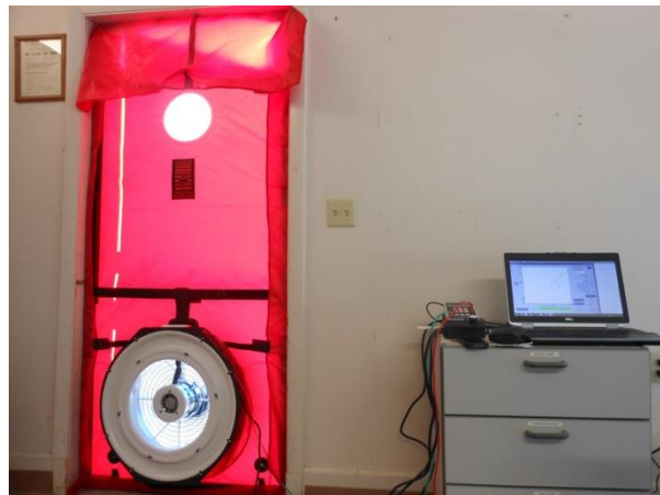
Figure 15: Blower door experimental setup at the Brunswick site performed on December 12, 2012. A blower fan is installed on the exterior door. The fan can generate pressure differences as high as 60 Pa. A computer is used to control the fan and data acquisition.
