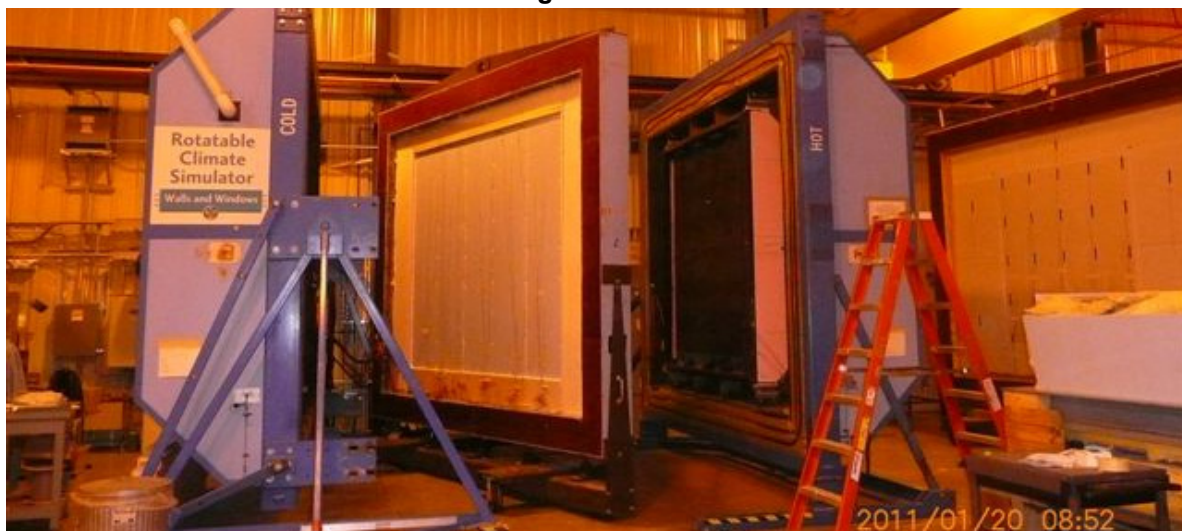
Figure 23: Hot Box Testing Chamber
