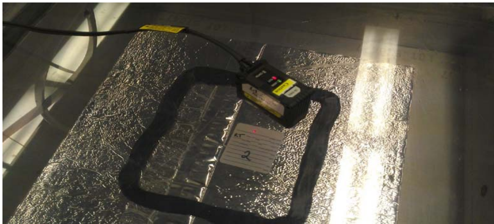
Figure 2. VIP within the vacuum chamber being measured for deflection using a laser
