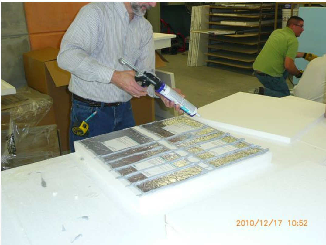
Figure 4: Construction of 2' x 2' x 3" VISE
