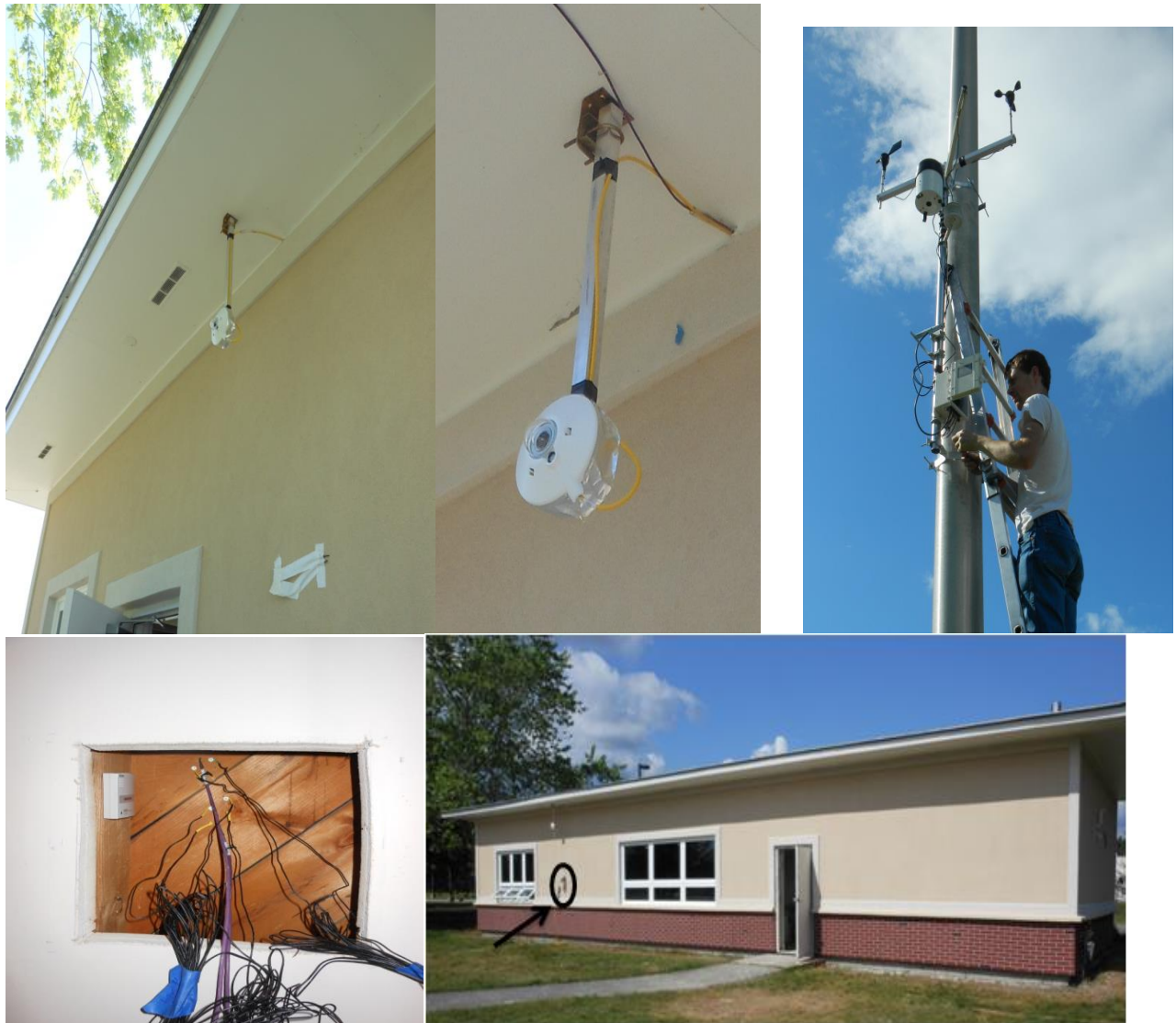
Figure 19: Pyronometer and weather station (top); Installed sensors in the west wall cavity and on the façade (bottom)
