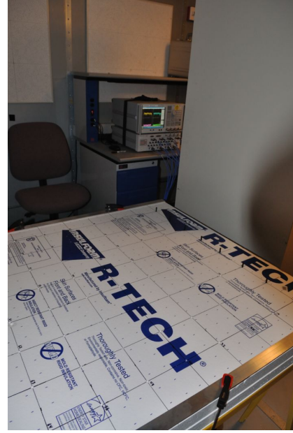
(b) Receive antenna array with a grid spacing of 13.5 cm
