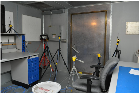
Fig. 4. Transmit antennas are placed in an irregular array to demonstrate that time-reversal does not require specific spacing, height, or even orientation of transmit antennas
