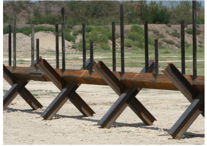
Fig. 2. Section of Modified Normandy Barrier (MNB)
