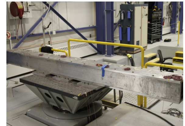
Surrogate PWR assembly on shaker table
