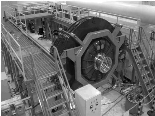
Fig. 3. The Mykonos II LTD, two 1-MA cavity voltage adder. The rail system can accommodate 20 LTD cavities.
