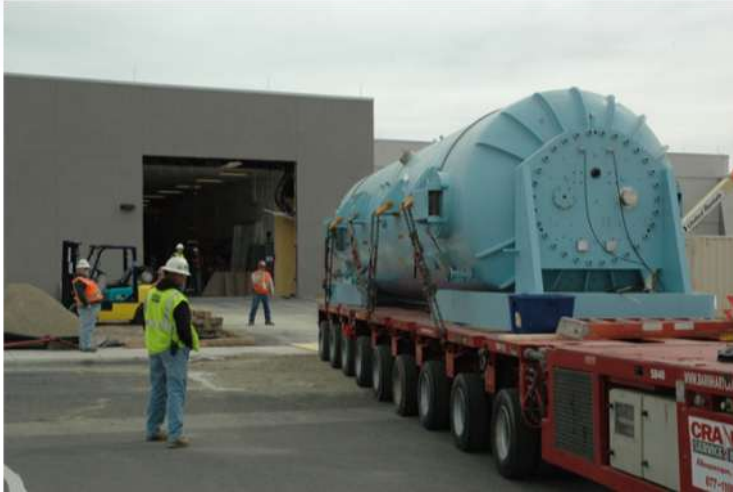
A special 72 wheeled vehicle with independent steering for each pair of wheels was used to move the Tandem accelerator
