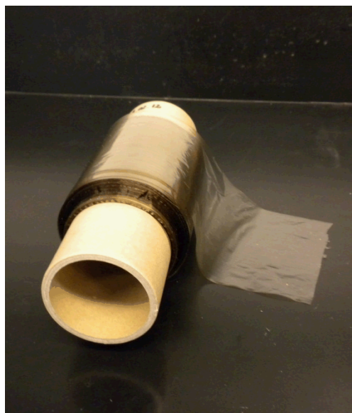
Extruded film with plasticizer Length ~80 m (3" wide)
