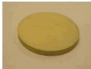
50 wt% Agl/50 wt% Glass, 500°C for 3 hr
