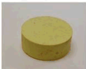
50 wt% Agl/50 wt% Glass 500°C for 3 hr
