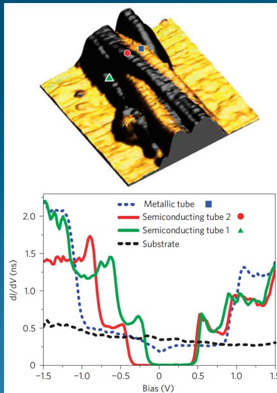
Asymmetric (w.r.t.  $E_F$ ) peak positions due to tube-substrate charge transfer.
