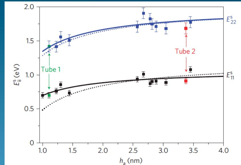
these reasons we provide empirical fits using  $E = E_0 - C_1 e^2 / (2h_a)$ , where  $C_1 = 0.52C_0$  for the  $E_{11}$  gap and  $E = E_0 - C_2 e^2 / (2h_a)$  with  $C_2 = 0.89C_0$  for the  $E_{22}$  separation (solid lines in Fig. 3). Note that
