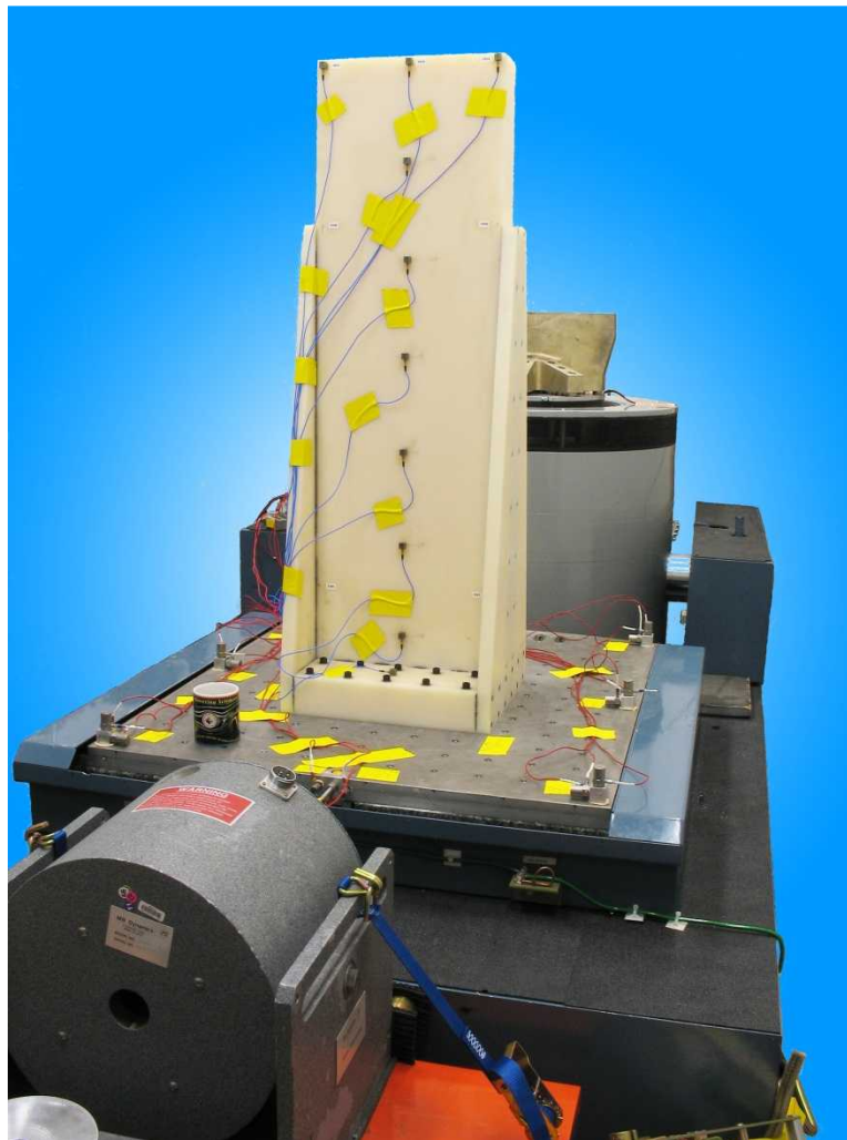
Figure 6 - Test Article Mounted on Slip Table with Portable Shaker
