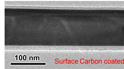
Carbon layer provides a large sea of electrons to activate the lithiation at the surface.
