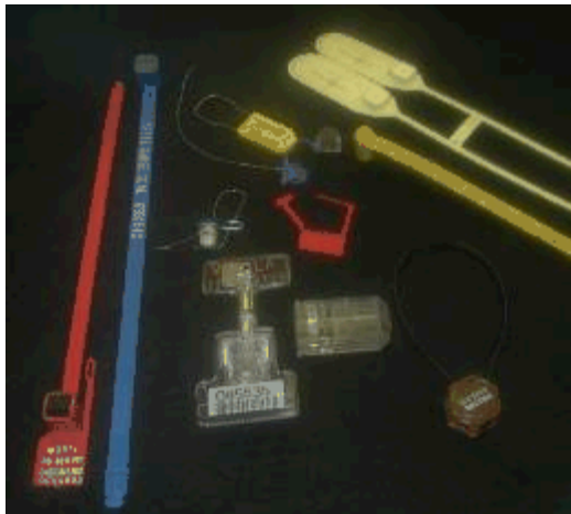
Candidate plastic seals for application of OSL taggant
