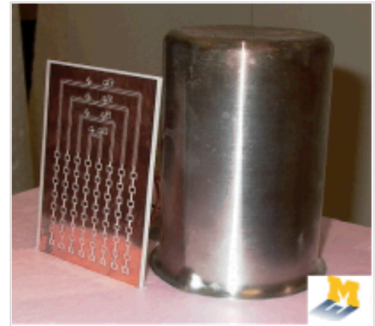
Totally passive ultrawideband (UWB) radiofrequency (RFID) tag
