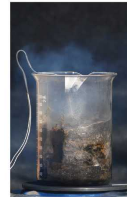
Decomposes and ignites before melting completes.
