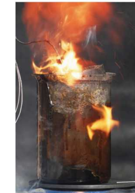
Decomposes and ignites before melting completes.
