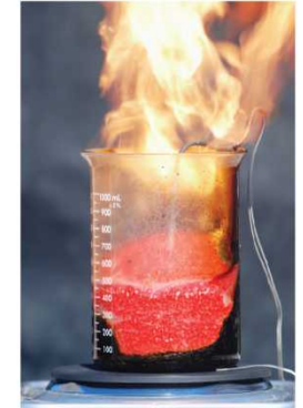
Does not slump as melting occurs, gases ignite in air.
