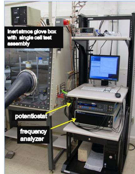
The ceramic foams are backfilled with conductive liquid and impedance tested. Molten salt electrolyte requires high temp (>370C) & inert atmosphere glove box.
