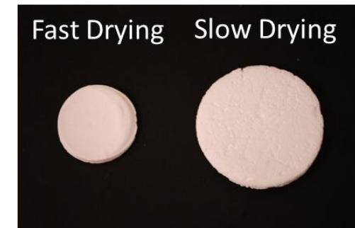
Slow drying leads to less shrinkage = higher porosity
