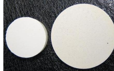
Separator must be flat and of an appropriate shape
