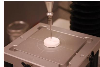
2 mm diameter post driven into sample. Fracture force measured.
