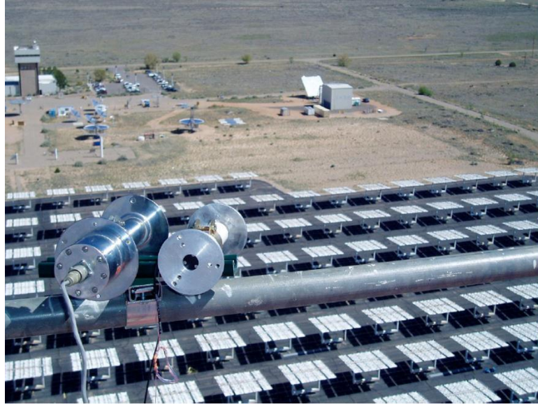
Figure 3: Eppley NIP (left) and Collimated LI-COR LI-200 (right) are aimed at a heliostat to test for response time.
