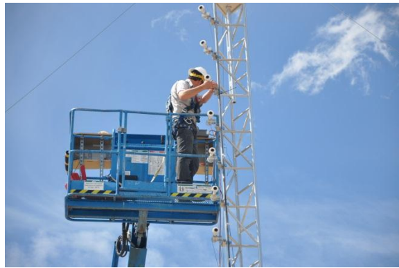
Figure 7: Technician aims sensor at a light source.
