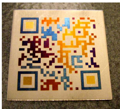
Figure 1. Example color QR code created in the surface of Ti. This Ti specimen was ~0.85 mm thick and 2.5 x 2.5 cm. This sample was irradiated in air, and it was not preheated before laser exposure. The color pixel size in this sample was 0.7 mm.
