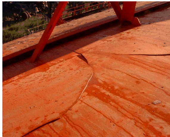
Figure 7. Example of cryogenic damage of steel ship decks from LNG spills
