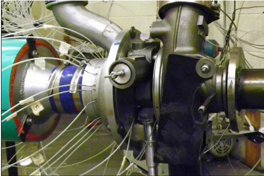
Fig. 7.1 Instrumented advanced MD turbocharger on flow bench
