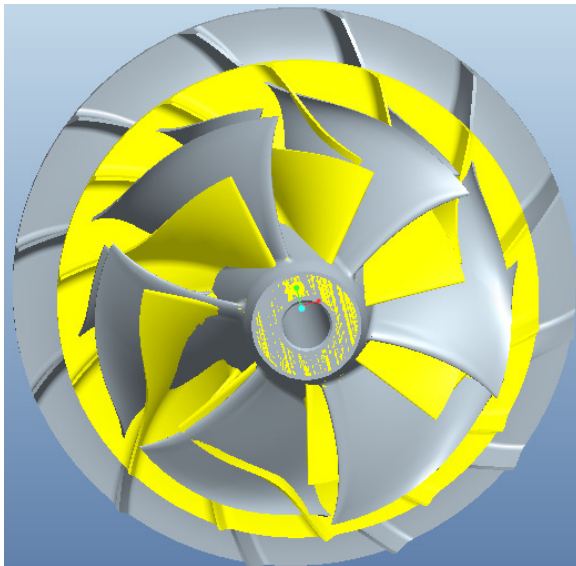
Fig. 9.1 Comparison of advanced MD (grey) and LD (yellow) compressor impellers
