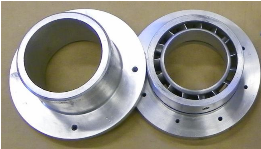
Fig.6.5 compressor insert for different casing treatment configuration
