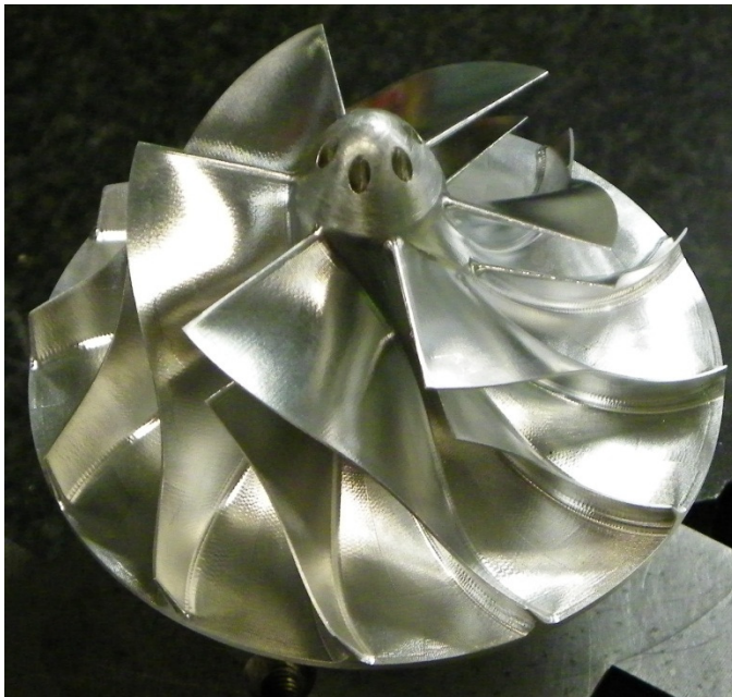
Fig. 12.14. Fabricated advanced MD2 compressor wheel with ruled surface
