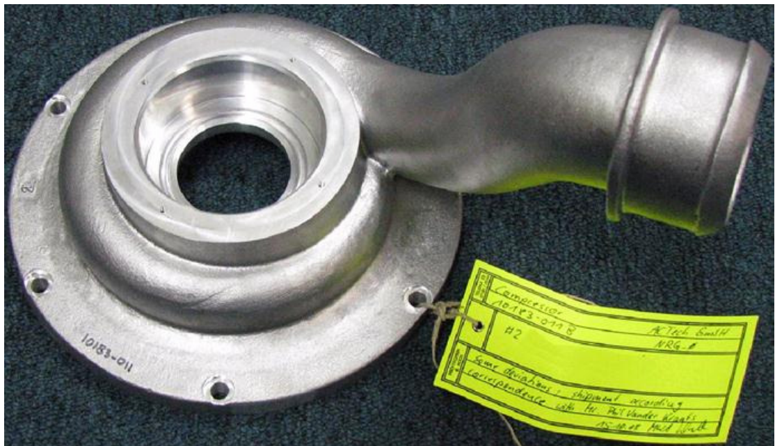
Fig.6.2 Prototype of advanced compressor housing with ultra-low solidity diffuser vane inserts (the vaned diffuser was later on replaced by active casing treatment)
