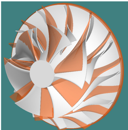
Fig. 3.1 Comparison of a conventional (red) and the advanced impeller
