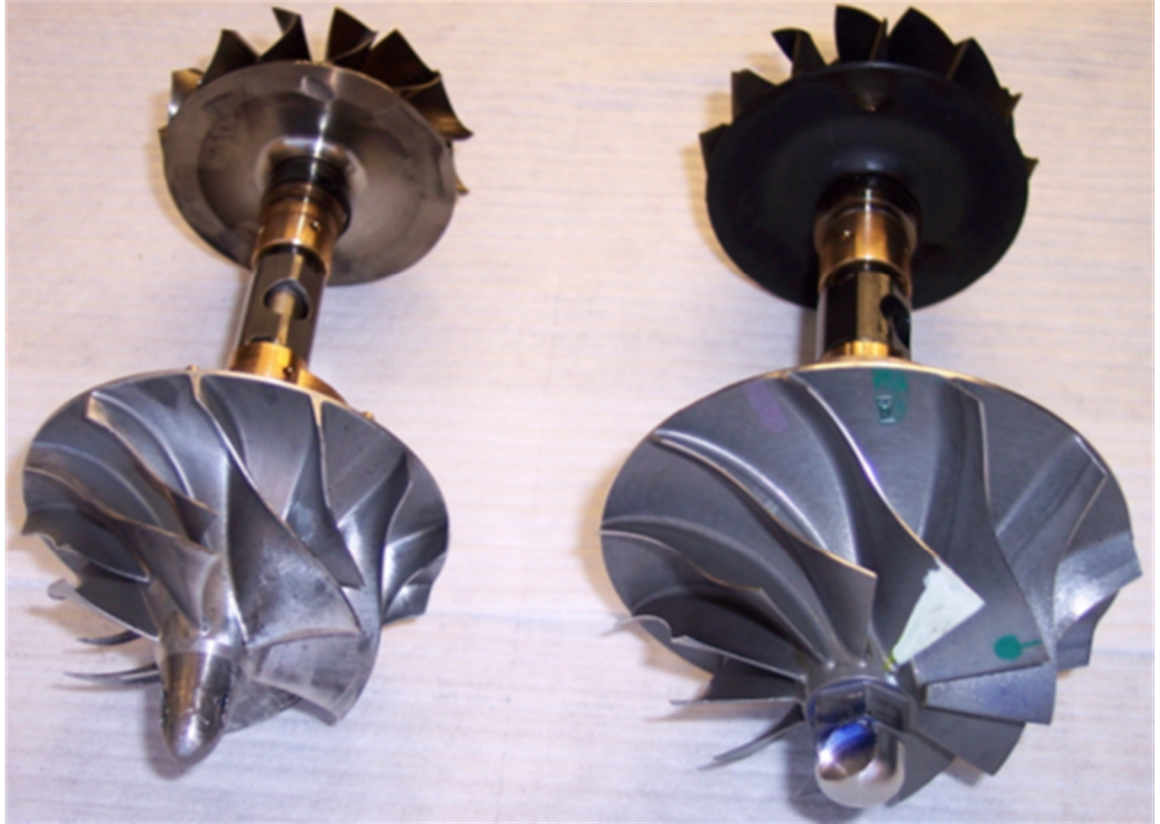
Fig.6.1 Comparison of advanced turbocharger (left) with conventional turbocharger wheels
