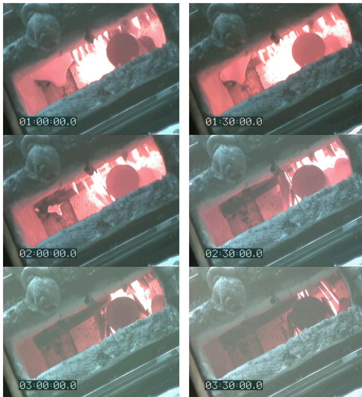
Figure 2. Video frames from the combustion of 45 kg of carbon fiber epoxy panels at regular half-hour intervals, as time-stamped.
