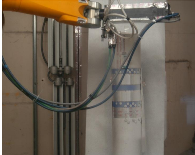
Figure 6, Cylindrical spray operation in progress for TP48. The first few layers of SASN appear white and completely cover the flyer plate and direct spray samples. This the same set up used for shot series TP49, which is the focus of this study.
