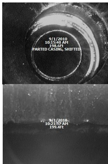
Figure 5. Camera shots showing parted casing (top: looking down well, bottom: sidewall image) just above collar at 60.8 m (199.5 feet) (courtesy DM Petroleum Operations Co.).
