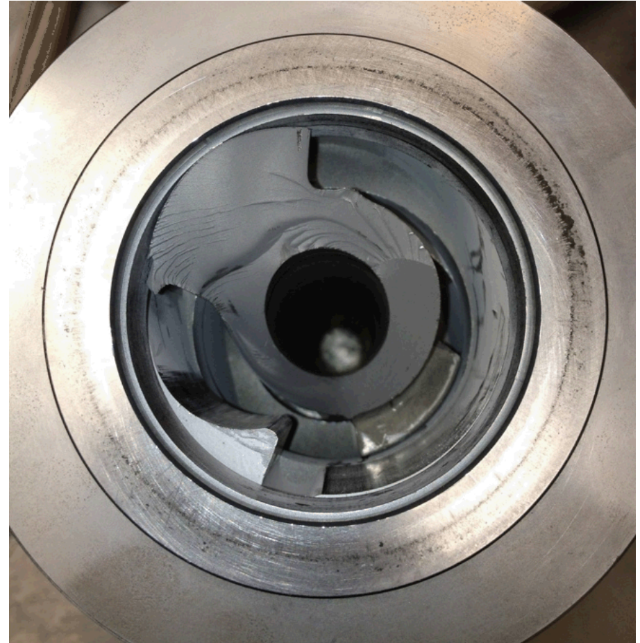
Brittle failure of A2 drive shaft
