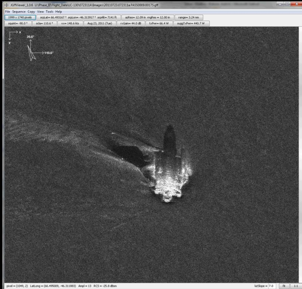
In one experiment in Greenland, radar reflectors were positioned in a snow drift to test radar penetration of the wet snow. This is a single image from a 1 foot resolution VideoSAR pass on a decommissioned early warning radar site that preliminarily indicates that the reflectors are visible.
