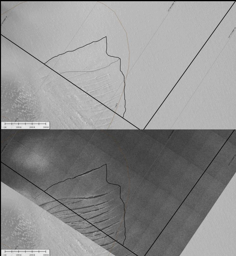
Data sets from the Nov 2011 deployment show that the CDR system detects all crevasses that are noticeable in the optical data.
