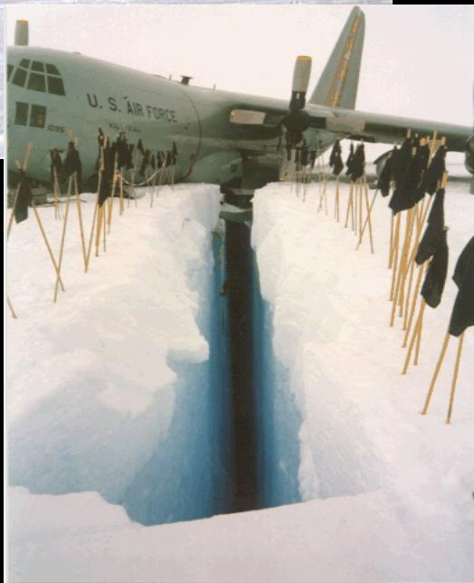
On November 16, 1998 the left ski of an LC-130 broke through an ice bridge that covered a crevasse. The crevasse was 10 feet wide and the ice bridge was estimated as 8 feet deep. The accident occurred near field camp on the West Antarctic Ice Sheet, 80 miles SW of Siple Dome Camp.
