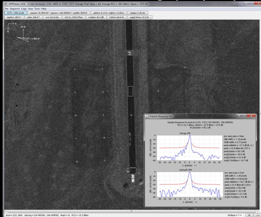
A large scale test range is located on Kirtland AFB. For remote testing corner reflectors are placed in low clutter areas – for a simple check of system IPRs.
